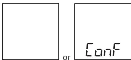
After configuration, the logger is ready to start recording, this is indicated in the display accordingly:
