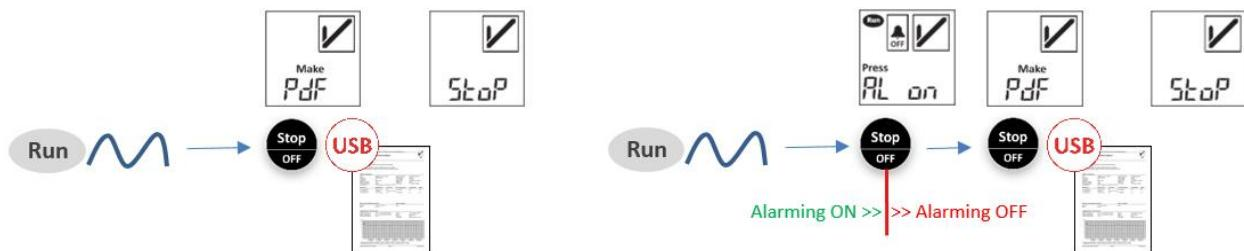
You can apply the two stop options mentioned above in parallel during the configuration (the logger can be stopped by one or the other method).
