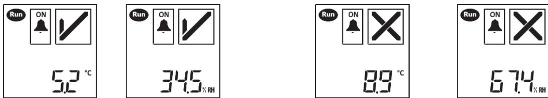
From this mode you get to the **stop mode** at the end of the monitoring period by stopping the logger via the configured stop option (via pressing "Stop/OFF" button for 2 seconds or USB connection).
