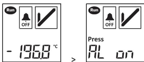
During the phase of "AL ON" on the display, it is possible to display the current measured value for 2 seconds by briefly pressing the "Stop/OFF" button.
