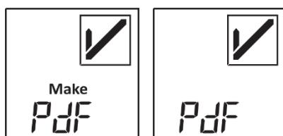
It disappears after the PDF report has been created by plugging the device into the USB port of a computer or retrieving the report via the Cx BLE Bluetooth® app. As a result, "StoP" appears on the display.
