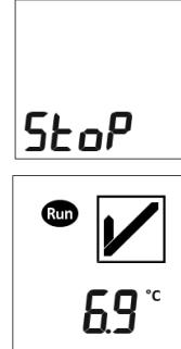
If a download is requested during operation ("Run Mode") the logger continues to run without any change in recording mode.
