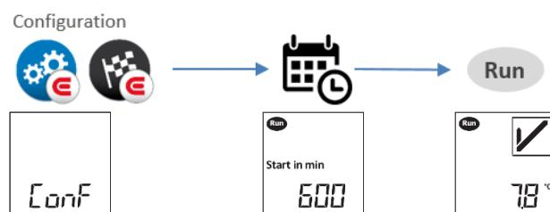
**CAUTION!** When re-starting or re-configuring from stop mode, **ALL RECORDED DATA** in the logger will be **DELETED** !
