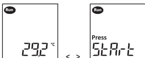
If a **temperature- or time-dependent delayed alarm activation** has been configured, a corresponding message appears in the display after the device is started:
