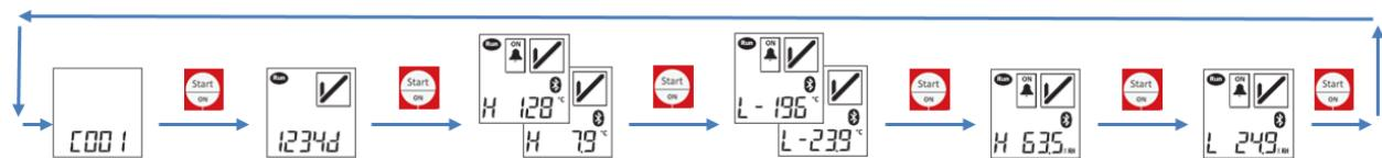
This step-by-step mode can be exited by briefly pressing the "Stop/OFF" button. If no button is pressed for 5 seconds, this is done automatically.
