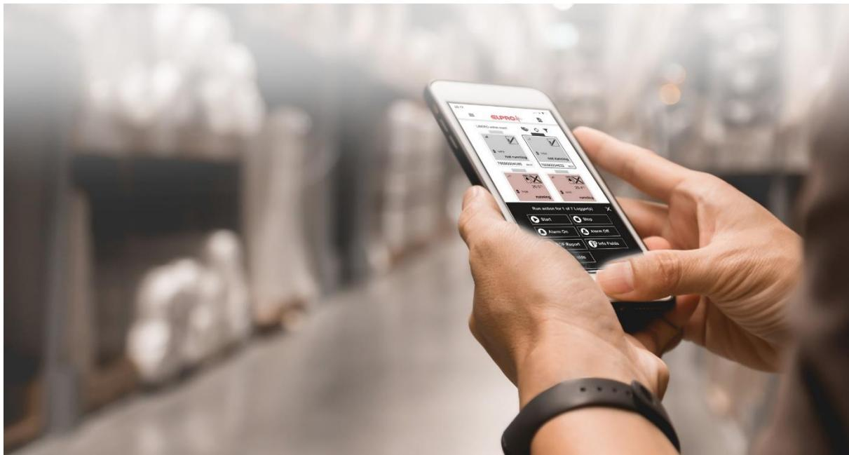
The ELPRO LIBERO Cx BLE app is a mobile app available for smart devices with iOS and Android operating systems. LIBERO data loggers with Bluetooth® Low Energy (BLE) interface are able to connect wirelessly to the app once installed on smartphones or tablets.
