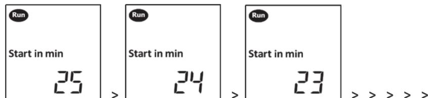
If a time delay was started, no operation of the logger is possible during this phase, the set delay time must be waited until the end.
