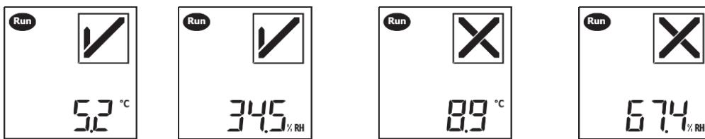
LIBERO CH-BLE alternatively displays the humidity value after briefly pressing the "Stop/OFF" button. Press the button again briefly to display the temperature value again.
