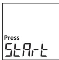
In this **start mode** the configuration of the device can be changed again if required. When plugged into the USB port of a PC, the device is automatically set to configure "ConF"-mode without the need to press any keys, and recognized by the liberoCONFIG software.
