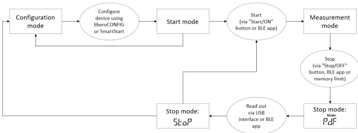
The following figure shows the sequence of modes if the "Alarming ON/OFF" function has been **configured** (also see chapter 6, section Alarm Conditions).
