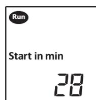
The delay time can be specified as any value (independent of the value of the selected logging interval), up to a maximum of 60 days.
