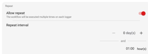
The repetition interval can be set in a range from a minimum of 1 hour to a maximum of 999 days.
